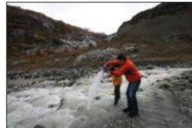
**Figure 12:** flow measurement of the proglacial stream by the salt dilution method.
