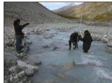
**Figure13:** classical measurement method for the flow of a proglacial stream: width and depth of the channel, flow velocity.
